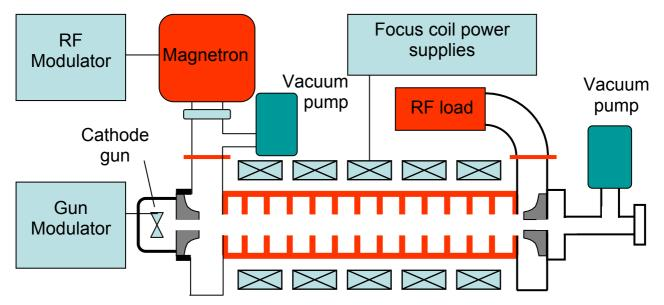
One of the features of our linac is that it is capable of producing single, variable width pulses on demand, in addition to the more usual repetitive pulses of  $\sim 4 \mu s$ . We achieve this by using a separate gun modulator. This is synchronized to the RF modulator and delivers a pulse to accelerate injected electrons during the much longer microwave pulse.
