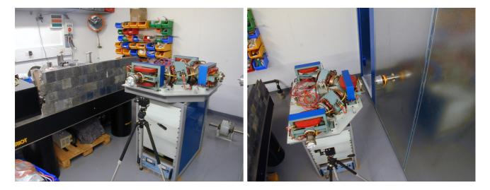
The immediate area outside of the beam end of the Faraday cage is dedicated to a beam switching magnet system. The rack below this is dedicated to DC magnet power supplies.
