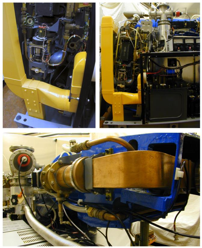
The linac's control system was extensively modified and matched with a new control software system. These will be described separately. However, we had decided early on in the project to provide convenient monitoring of the pulsed beam, both of its spatial position and of its temporal profile. This is achieved by placing a thin ( $\sim$ 1-2 mm) Suprasil silica disc at the output of the beam.
