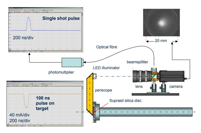
The lens/camera/beamsplitter can be rotated through +/-90 degrees and the 'outputs' of any of the three beam lines can thus be monitored.
