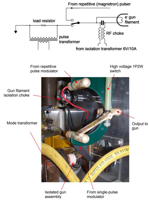
The gun modulator is based around somewhat dated, but effective thyratron switches (shown on the right); we had acquired several such switches over the years, and this approach was thus extremely cost-effective. Similarly, the output pulse transformer was 'to hand' and we were thus able to develop a novel type pulse generator to deliver many tens of kV at variable pulse widths.
