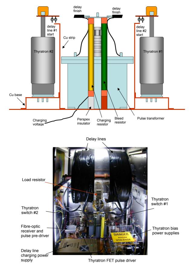
The machine's original magnetron modulator was not tampered with, other than relocating the main output pulse transformer. Its high voltage output pulse was guided to the magnetron and to the gun switch within insulated trunking (actually plastic trunking intended for bathroom ventilation systems!). Images of the radiofrequency source and the microwave output load are shown below.
