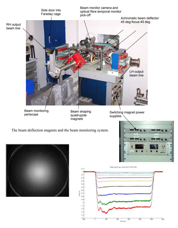
Such a beam monitoring arrangement is just fine when performing beam alignment prior to an experiment. However, when the periscope is removed, the operator would be 'blind' to the delivered pulse. To overcome this, a beam charge monitor is placed in the accelerator output beam line.
